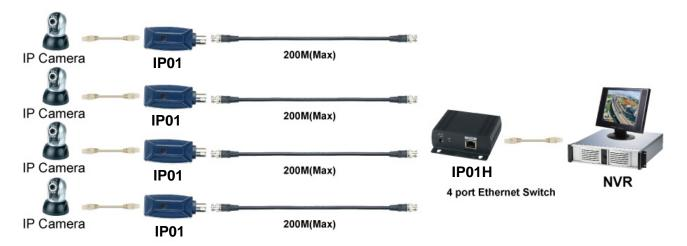
Caution: IP01H unit with BNC male terminator at channel 2, 3, 4. Do not remove the terminator if you do not use these channels. Otherwise, it will cause this Switch not working.
